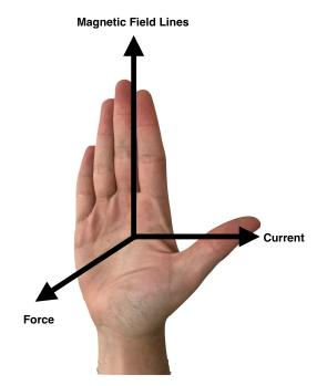
Finding the direction of the force between two wires
